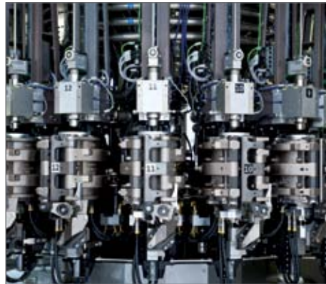
Modern stretch blow-molding machines can produce up to 81,000 bottles per hour.
