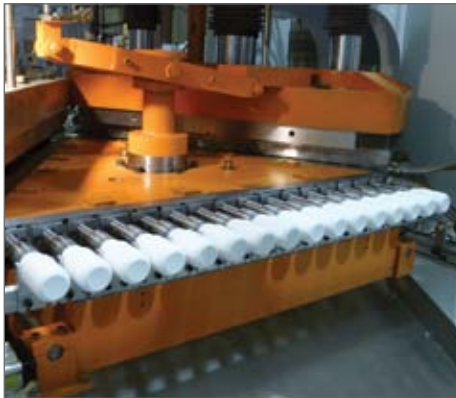
Plastic injection molding brings compressed air into contact with consumer good product containers.
