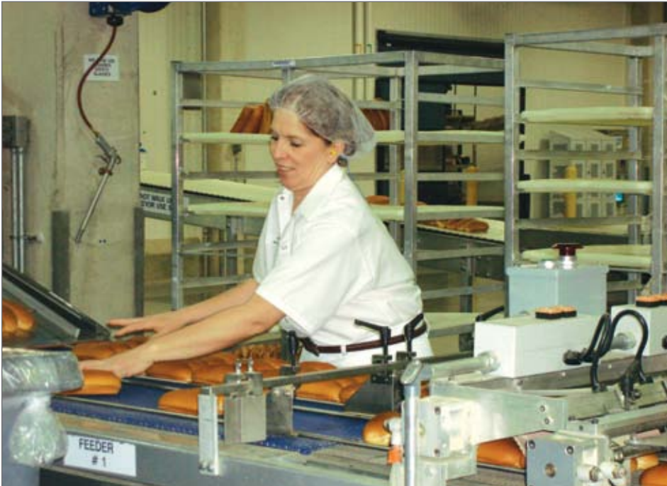
"Direct-Contact" application using oil-free compressed air to blow-off crumbs in a commercial bakery.
